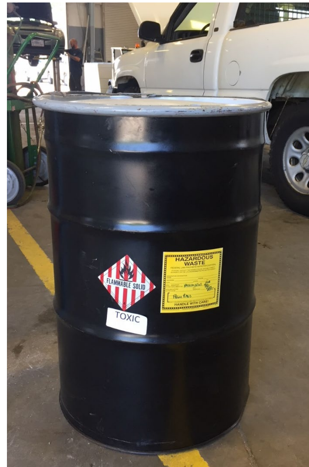
Properly labeled hazardous waste container.
