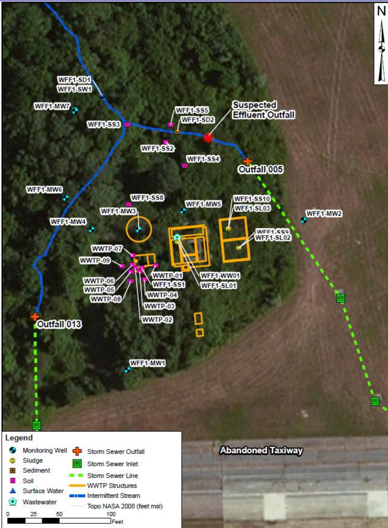
Figure 5: Old WWTP Sampling Locations
