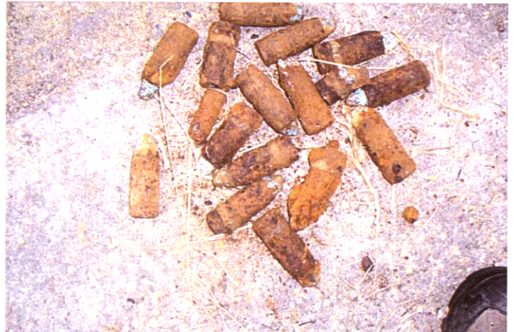
20mm/30mm items treated during Demolition
