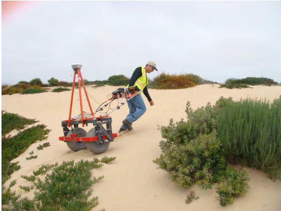
Figure 3-4 Geophysicist Performing DGM Surveys Using the EM61-MK2
