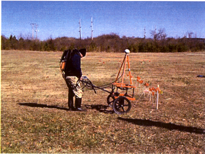
Geophysical Prove-Out using EM-61
