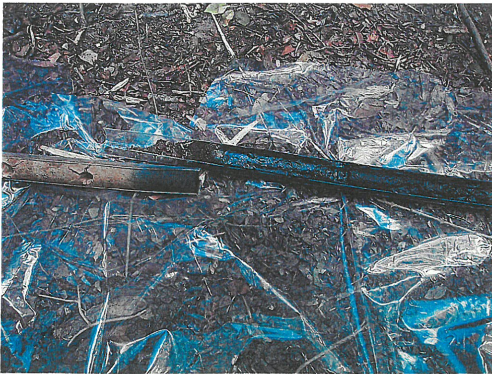
GeoProbe Soil Boring SB-CDL-01 with transition from reddish brown silty sand to contaminated black material at approximately 7.5 foot depth in 4' to 8' boring interval shown to the left. The 8' to 12' boring interval is shown to the right. The water table is within 0.5' of the visual transition—in the upper most portion of the core interval shown to the right of the photograph.
