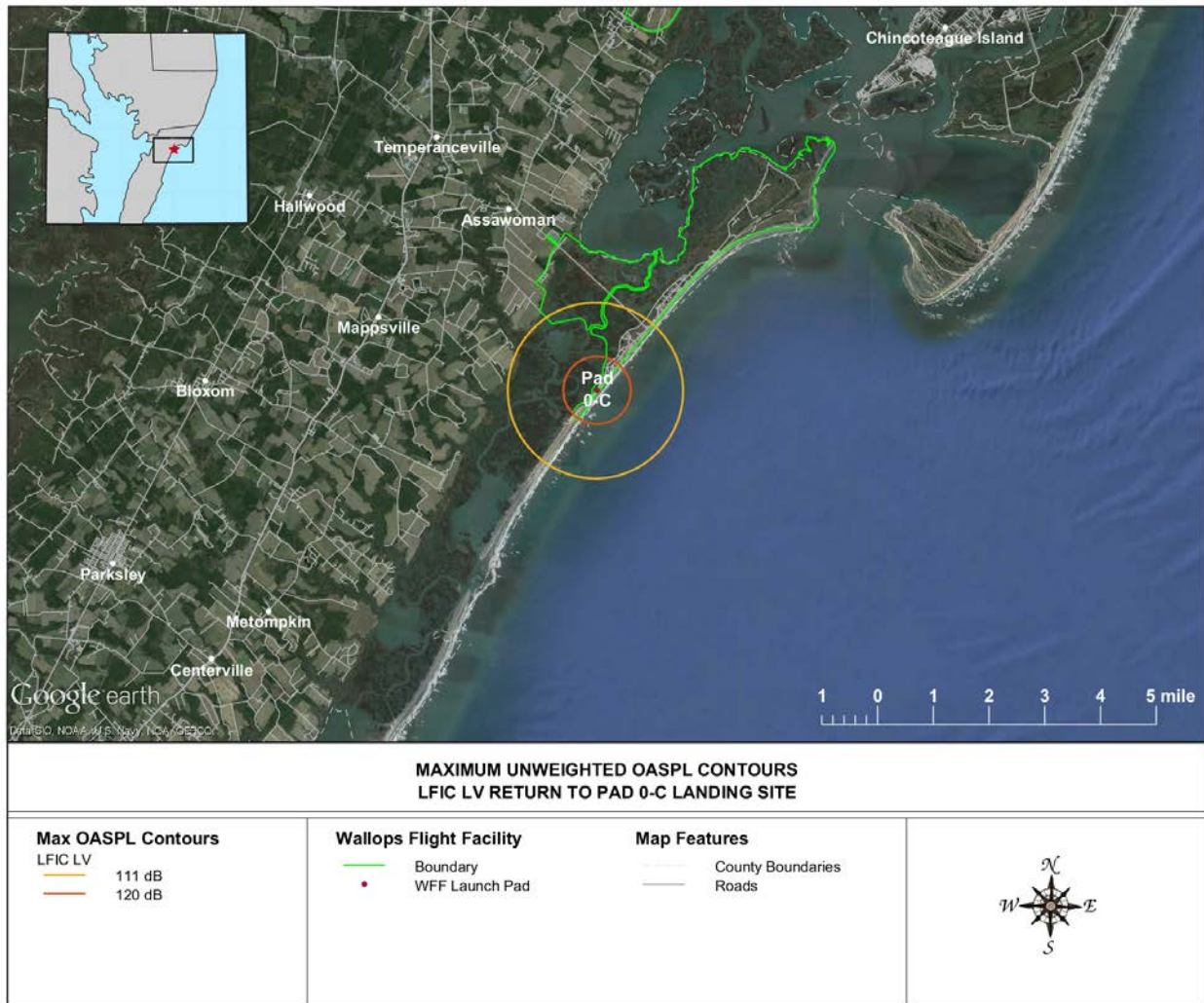
Figure 3. Maximum unweighted OASPL ( L_{max} ) contours for a LFIC LV return to the Pad 0-C landing site
