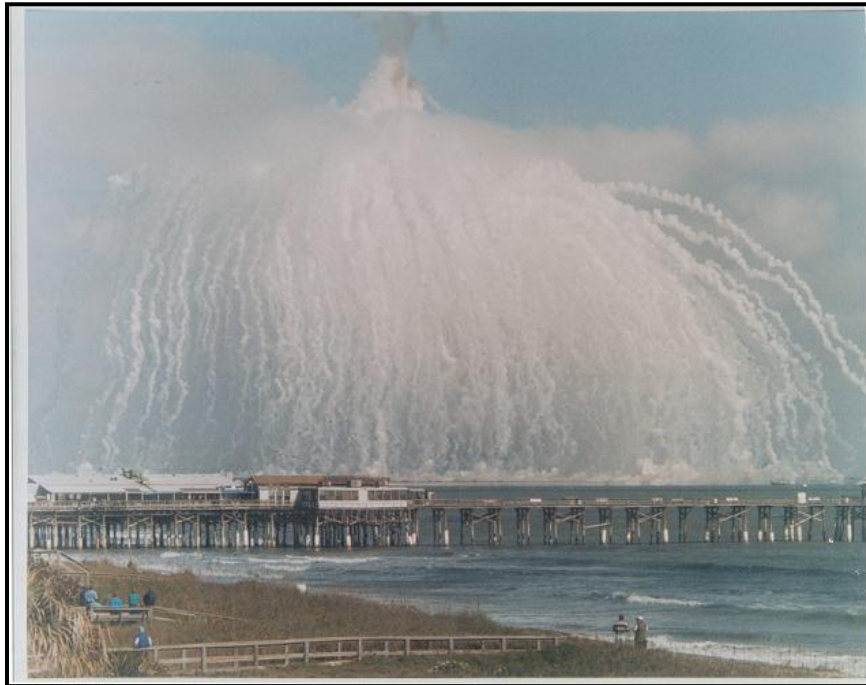
Figure 5-8. Trails of Toxic Exhaust From Burning Delta II 7925 Propellant Fragments that Fell to The Ground and Continue Burning.
