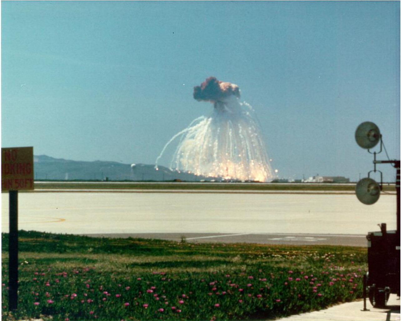
Figure 5-9. Solid Propellant Conflagration Cloud (White) and Liquid Hypergol Deflagration Cloud (Red) Formed When the Titan 34D-9 Vehicle Exploded at Vandenberg AFB.
