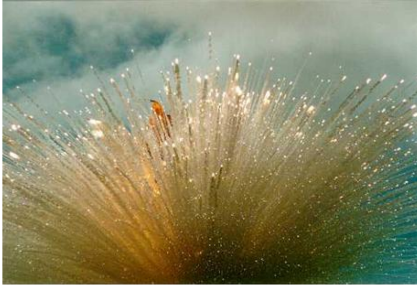
Figure 5-7. High Velocity Burning Propellant Fragments from a Delta II 7925 Solid Rocket Motor Explosion 13 Seconds into Flight.
