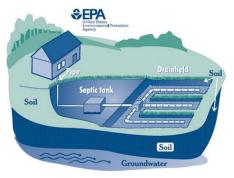
Septic tanks can be overloaded with wastewater, which can cause two problems. An abundance of water can disturb the sludge at the bottom of the septic tank and move it to the drainfield. This may clog the drainfield and prevent wastewater from filtering through the soil properly. In addition, large volumes of water may not be able to infiltrate the soil quickly enough, regardless of whether or not the
