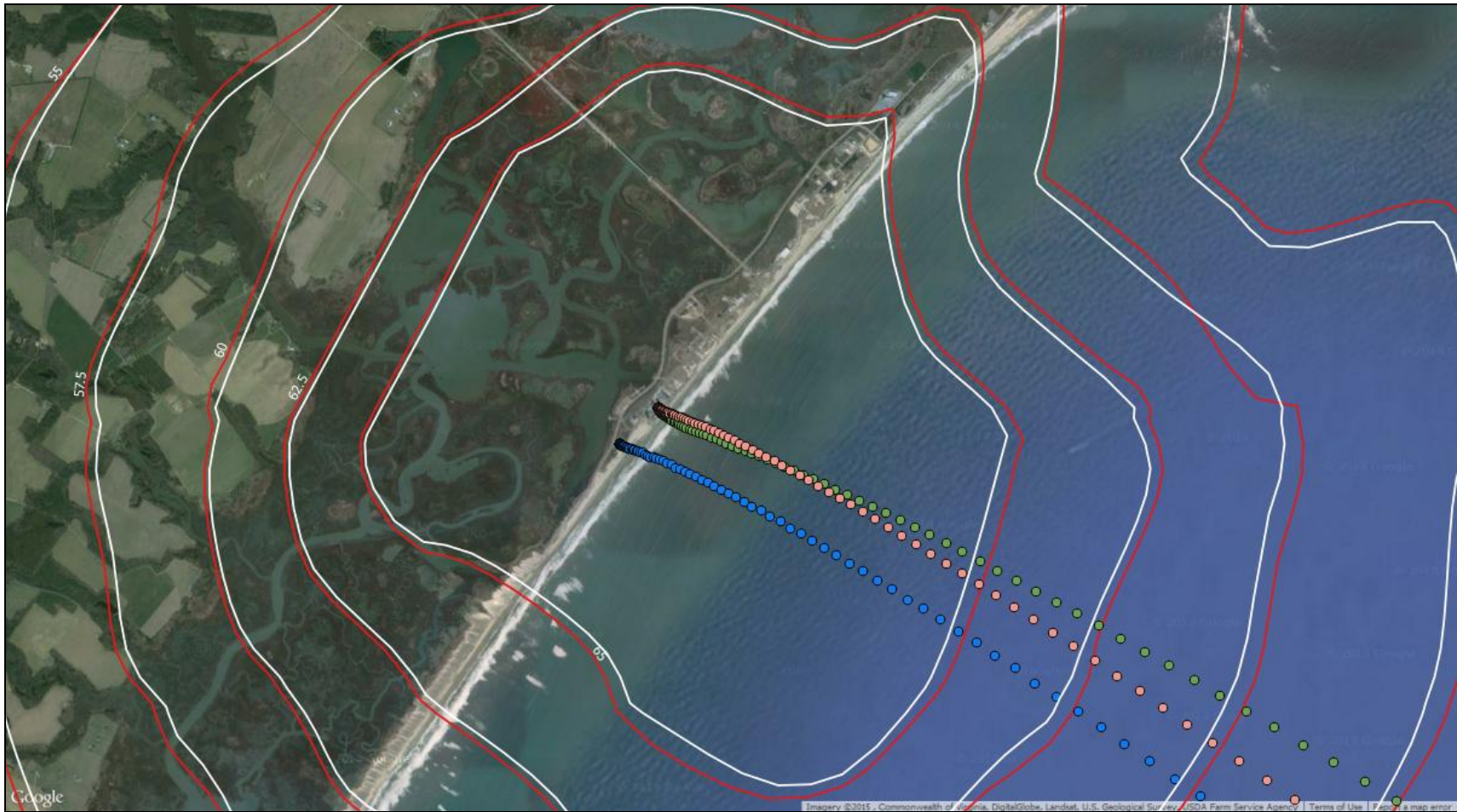
Figure 3-2: Day-Night Level Comparison of No Action (White Line) and Proposed Action (Red Line) Alternatives Note that the 65 dB Contours are the Innermost Shown (Source: ICF, 2015)
