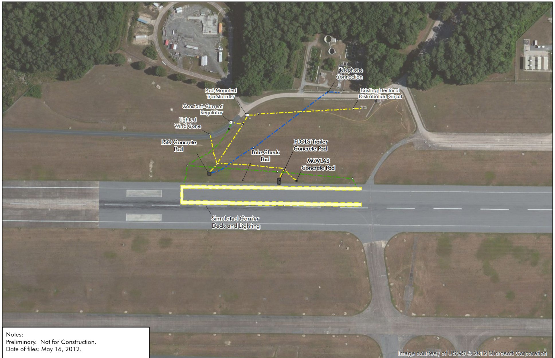
Figure 2-14 Runway 10: Proposed Modifications Wallops Flight Facility
