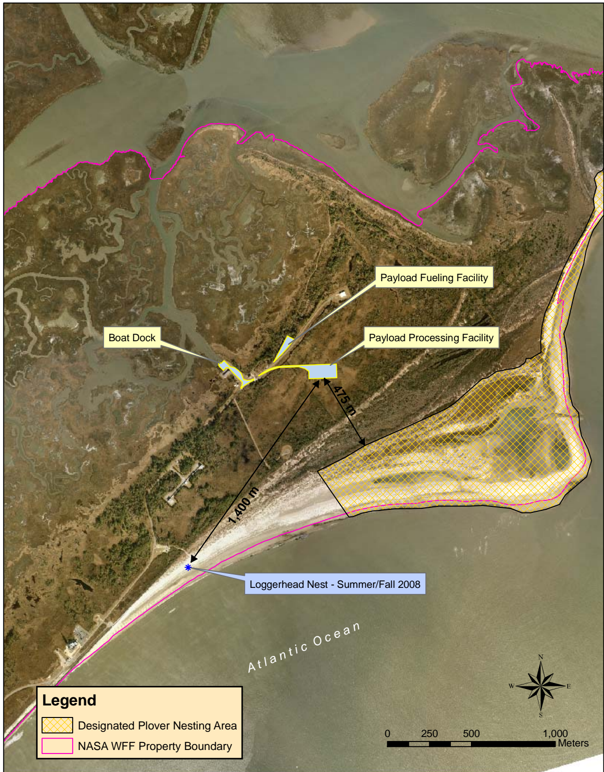
Figure 1 – Proposed Facility Construction on North Wallops Island
